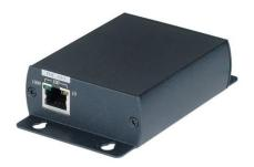
IP04 is a POE repeater to extend power and data an additional 100meters. Multiple units are allowed for longer distance, eliminating the need for additional switches, hubs and expensive fiber installations. It compliant with standard POE IEEE802.3af.
